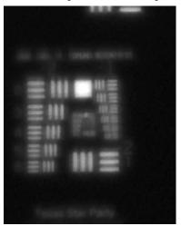
SCT with a x3 barlow operating at f30 and a video camera for image capture. Using the "lucky imaging" technique he captured many two thousand frames, selected the best 100, and then aligned, stacked and sharpened the result using Registax 6. An example resulting image is shown here.
