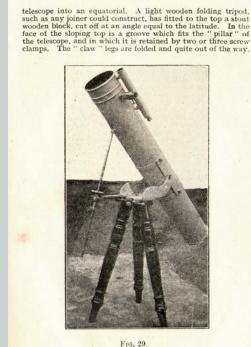
When it is desired to use the telescope for terrestrial views, it can be detached by unscrewing the clamps and set on its own feet. The above devices are quite successful with refractors up to about 4-in. aperture.
