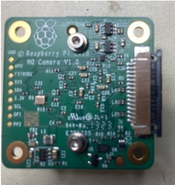
Locking tab in open position
